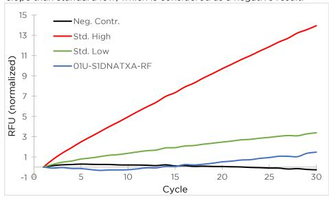
Image: Kinetic evaluation of RNase activity monitored on a real-time PCR system. Concentration of RNase A standards are 0.1 pg/µL for standard low (Std. Low, marked in green) and 0.4 pg/µL for standard high (Std. High, red). PCR-grade water is used for negative control (Neg. Control, black). Samples of 01U-S1DNATXA -RF are used to test RNaseactivity of the product (blue).
